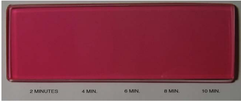
Figure 3b – Adhesive with Red Dye without UV Stabilizer Exposed to UV Light in 2 Minute Intervals
