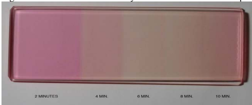
Figure 3b – Adhesive with Red Dye without UV Stabilizer Exposed to UV Light in 2 Minute Intervals
