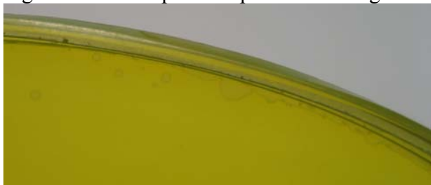
Figure 4b – Example of Separation During Curing Process
